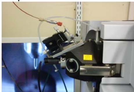
Figure 2: the nanospray probe source is installed at one of the windows of the Apollo source. A camera is also mounted to facilitate optimizing the nanospray emitter position with respect to the MS inlet, and also the quality of the spray.
