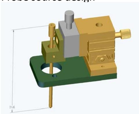
Figure 1: The probe source design. The nanospray probe, the part with the largest dimension in the source, is about 10 cm in length.
