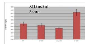
Error bars represent 1 standard deviation from the mean value of data from triplicate runs. Good correlation between peak width and both XITandem score and #unique peptides was demonstrated. The substantial improvement due to heating the column system and sheath gas is expected to further improve with complex samples.
