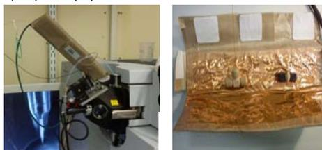
Figure 3: For the heated column and sheath gas experiments, the trap column, filter, analytical column and sheath gas tubing were enclosed in the “Butterfly heater mounted close to the source.
