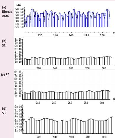
(a) to (d) are the deconvoluted results of the Hadamard multiplexed sprays experiment. (a) shows the binning of the MS results superimposed on the raw data. (b) to (d) are the deconvoluted results assigned to the corresponding sources. When compared to the relative intensities of the TIC of sequential spray data, it is clear that the deconvoluted multiplexed data match the sources correctly.
