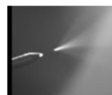
PST-mTip-50: Extremely stable spray for methanol from top: 3 \mu L/min, 8 \mu L/min and 26 \mu L/min
