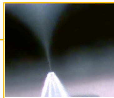
A PST-polytip coupled without a fitting to a SureSpray™ nozzle creates a robust, clog-free spray with negligible dead volume. Sheath gas can be used with the nozzle with sheath gas flow channels.
