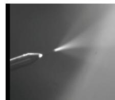
PST-mTip-50: Extremely stable spray of methanol from top: 3  $\mu$ L/min, 8  $\mu$ L/min and 26  $\mu$ L/min
