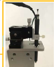
Insert the probe into the 3-D positioner and adjust the tip position from the MS inlet
