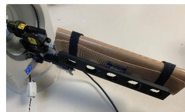
Butterfly heater for the EasySpray source. Suitable for the Pharmafluidics columns and any other columns.
