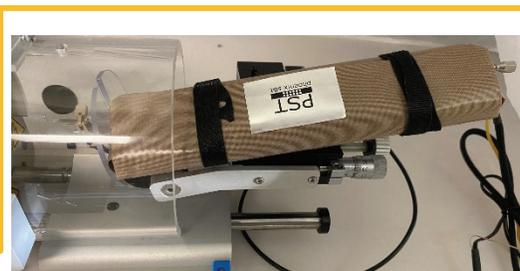
**Butterfly Heaters** -The heater surface is electrically insulated and the mounting support is available for the Easyspray and Nanoflex sources
